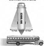
May use in conjunction with the left and right side standard (flat) mirrors to obtain the desired visibility
